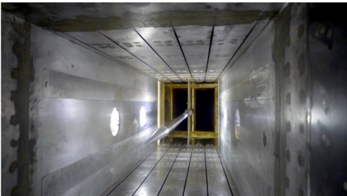
图 5 短轴探管(DJZ-T) Fig.5 Short centerline probe (DJZ-T)
